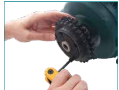
REMOVING A TAPER LOCK BUSH
