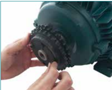
TIGHTEN SCREWS FINGER TIGHT
