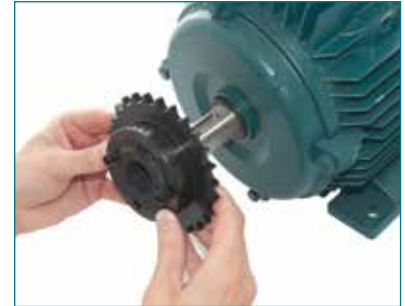
INSERT SCREWS AND LOCATE ON SHAFT
