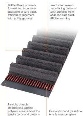
tensile cords and protects them from containments and mechanical damage Helically wound glass-fibre tensile member gives high tensile modulus and excellent fatigue life
